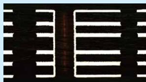
厚銅基板断面 X-section of Heavy-Cu PWB
