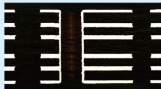
厚銅基板断面 X-section of Heavy-Cu PWB
