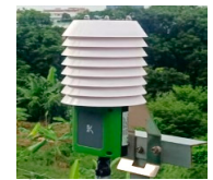
Outdoor weather observation station
