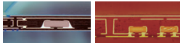
[Mass production of product] [Development product] Plate Solder connection embedded PCBs connection embedded PCBs
