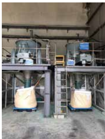
Photo 2: Equipment for recovering copper carbonate in Vietnam Plant
