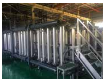
Photo 1: Equipment for recovering metallic copper in Vietnam Plant
