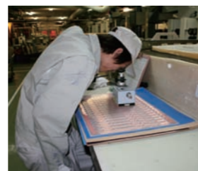
Outer layer circuit pattern process
