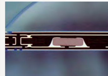
Photo showing cross-section of an embedded PWB
