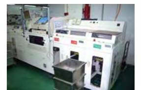
Four-terminal electric checker
